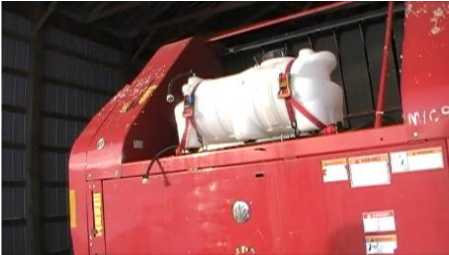
Dalmeny field day January 22 Viewing adaptations made to baler to apply hay preservative
